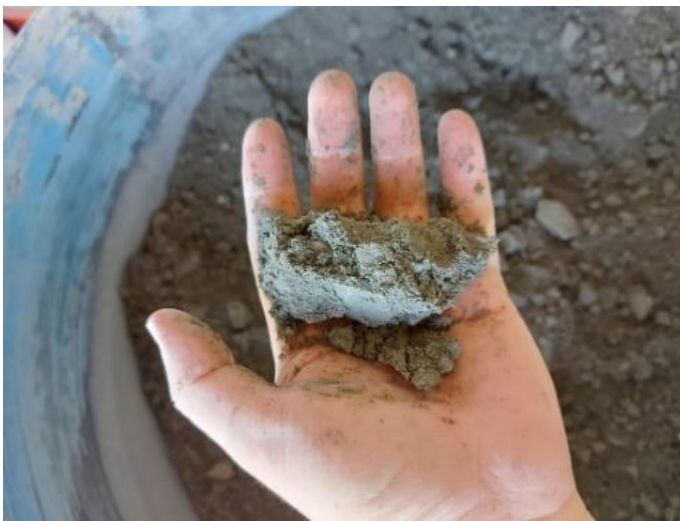
Figure 1 Consistency of RCC mixture
