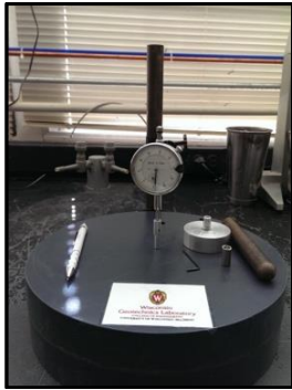
Figure 6 Testing equipment for geocomposite thickness measurement
