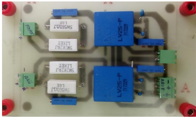
Fig. 2. The voltage reading card. (a) The open-circuit diagram. (b) Final form of the card.
