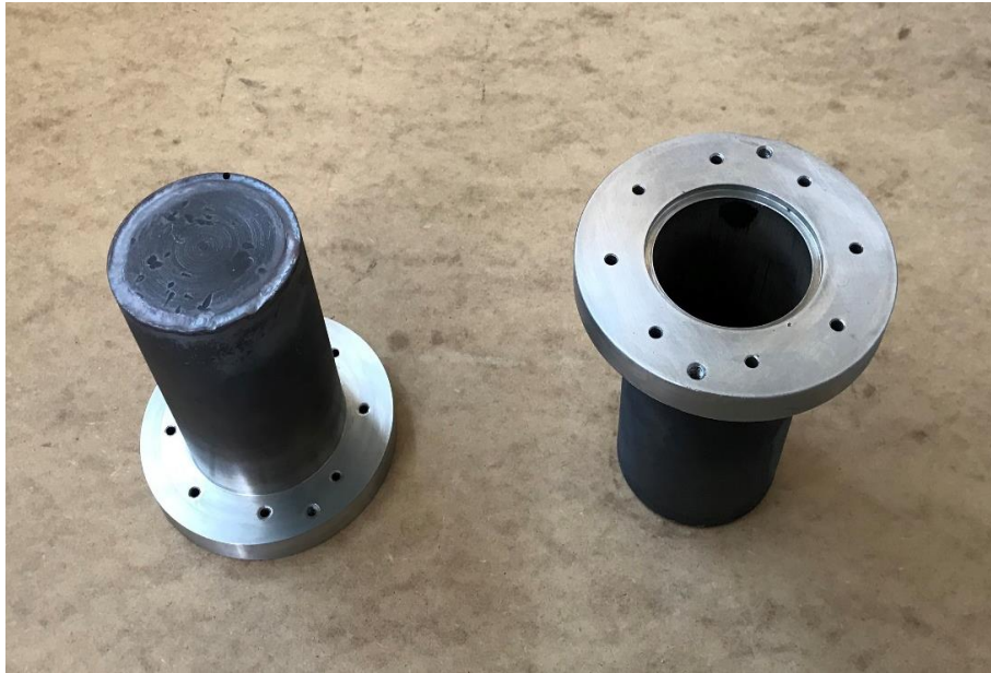
Figure 10. Schematic view of the manufactured displacer cylinder
