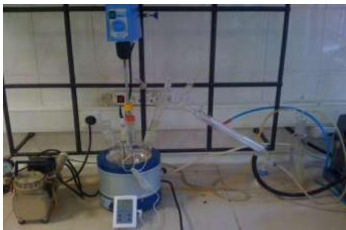
Figure 1. Experimental setup used in the synthesis of butyl-glycoside and alkyl polyglycosides.
