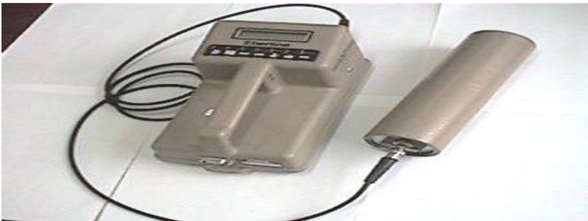
Figure 1: ESP-2 Rate meter and SPA-6 scintillation detector, Eberline (18).
