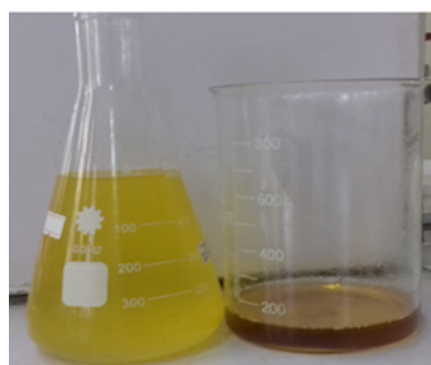
Right, biodiesel and glycerin after separation
