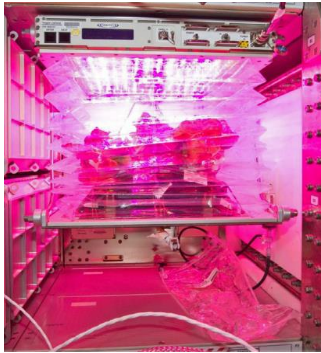
Figure 9: "Veggie" Vegetable Production Unit on the International Space Station.
