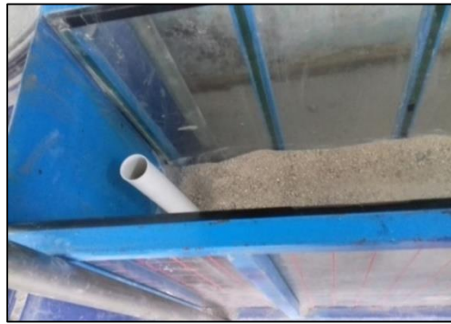
Figure 3. Positioning of the PVC pipe inside the sand in Model 4.
