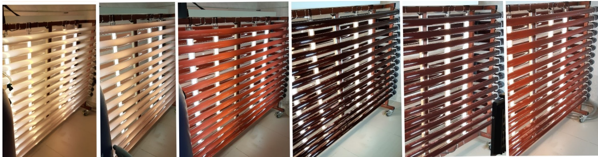
Figure 2. Porphyridium cruentum culture at tubular PBR (left to right: 1 st day, 7 th day, 14 th day, 24 th day, 34 th day, 44 th day).
