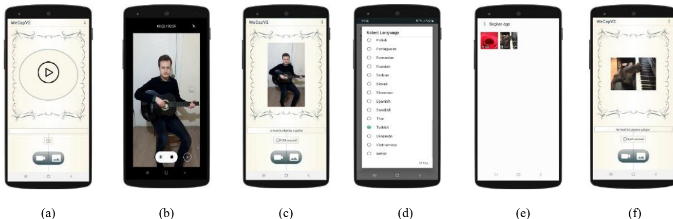
Figure 3. Android application: the homepage is given in (a), a live video is captured in (b), the generated caption with video is shown in (c), language options, gallery, and the translated caption are given in (d), (e) and (f), respectively.
