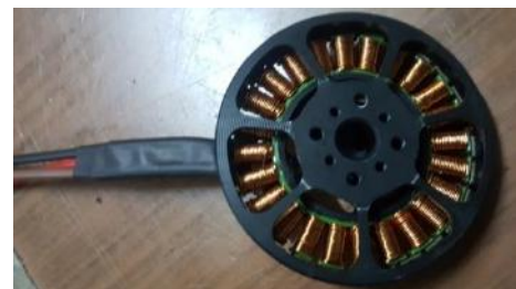
Figure 11. Winding stage and final picture of produced BLDC motor.
