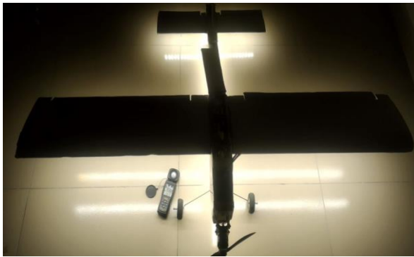
Figure 14. Display of the brightness measurement of the UAV
