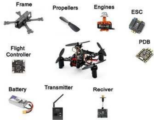
Figure 2. Main Components and Systems of UAV
