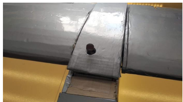
Figure 13. The representation of the external surface sensor on UAV
