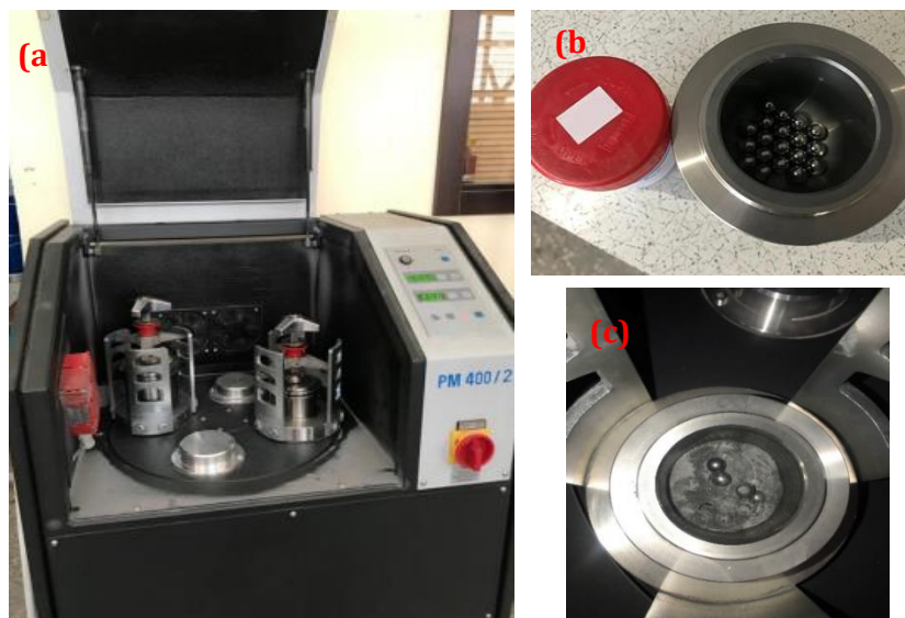
Figure 1. Schematic of The Mechanical Alloying Process (A) Retsch PM400/2 Ball Planetary Mill, (B) 125 ml WC Grinding Jar With 10 Mm Diameter WC Balls, (C) Addition of 1% Zinc Stearate
