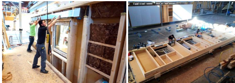
Figure 7. Metal ventilation duct included within the wood frame prefabricated facade panel (4RinEU, 2022)
