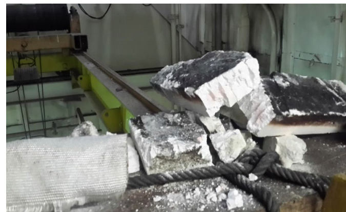
Figure 6. The parts which fell off funnel loop
