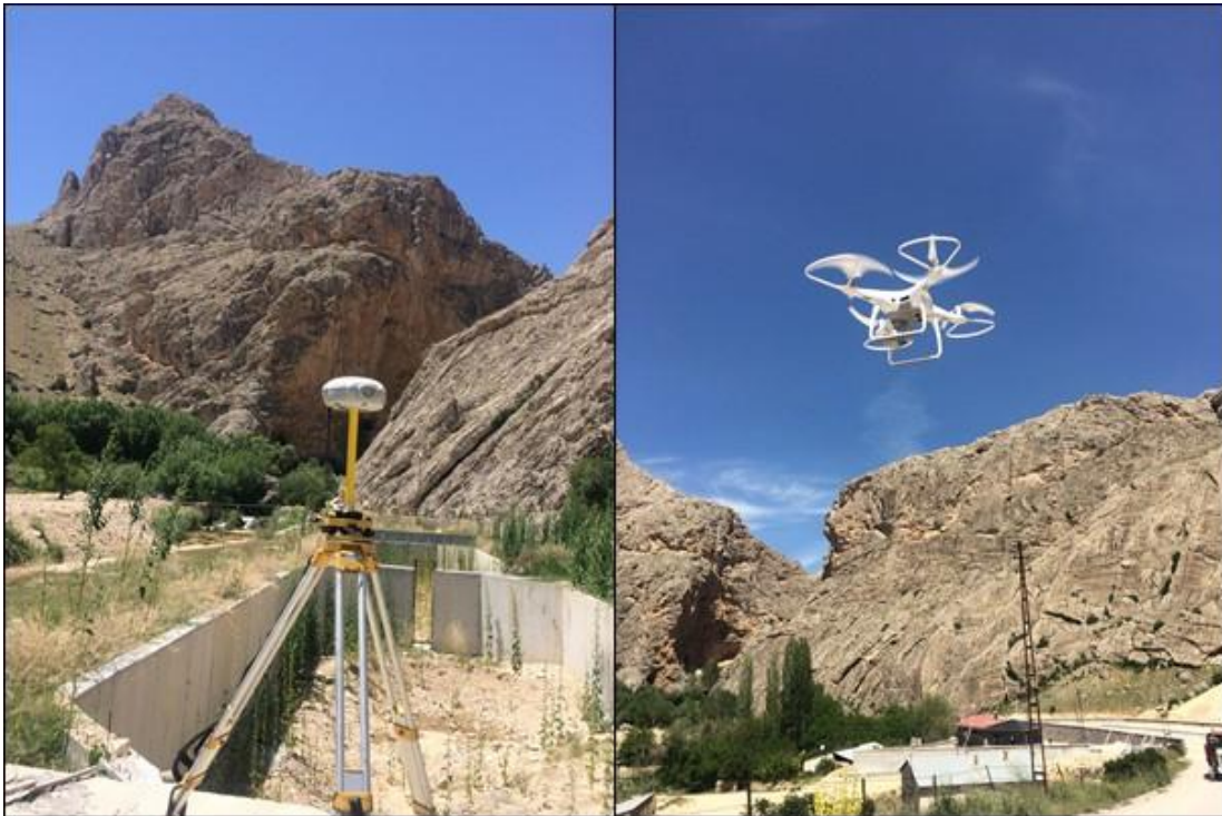
Figure 2. DJI Phantom 4Pro model UAV and CHC X91 model RTK-GNSS receiver used for data acquisition
