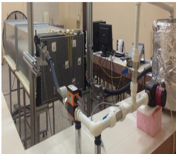
Figure 1. Actual and schematic view of the experimental system (1-storage tank 2-circulation pump 3-ball valve 4-flow meter 5-compact heat exchanger 6-recycle line 7-data logger 8-air flow channel 9-fan 10-computer)
