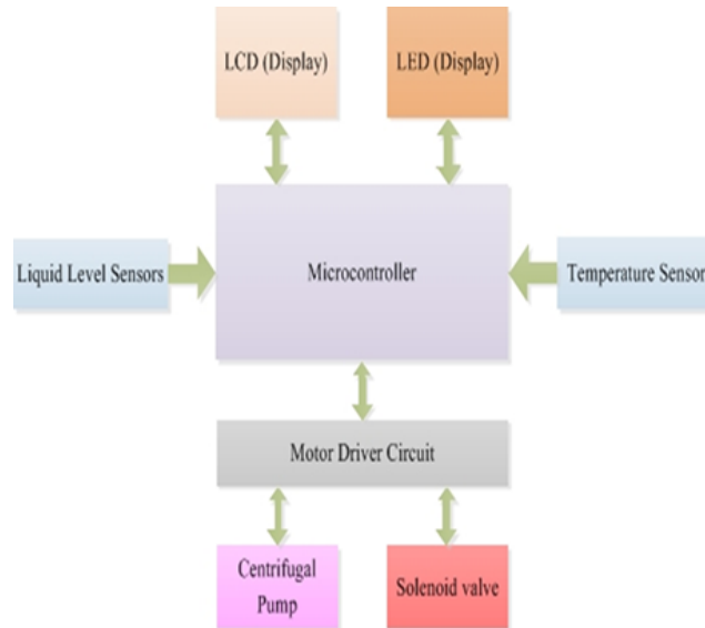
Figure 2. Block diagram of the mechatronic liquid level measurement system
