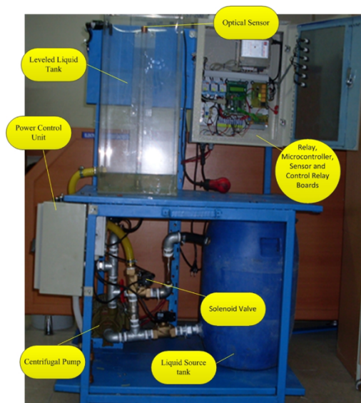
Figure 6. Mechatronic liquid level measurement system
