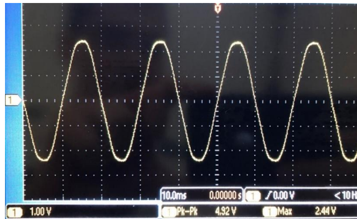
Figure 6. Fault current in the system with R-SFCL
