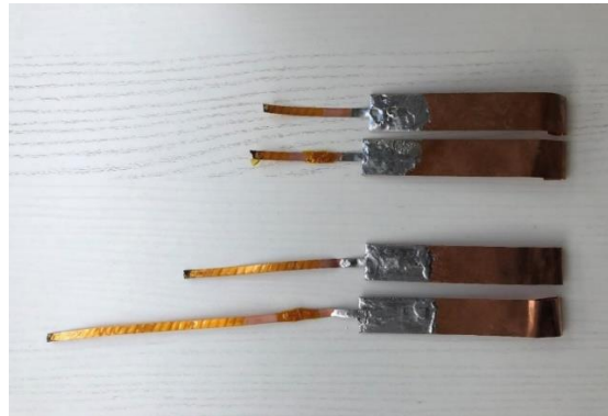
Figure 10. Damaged superconducting tapes
