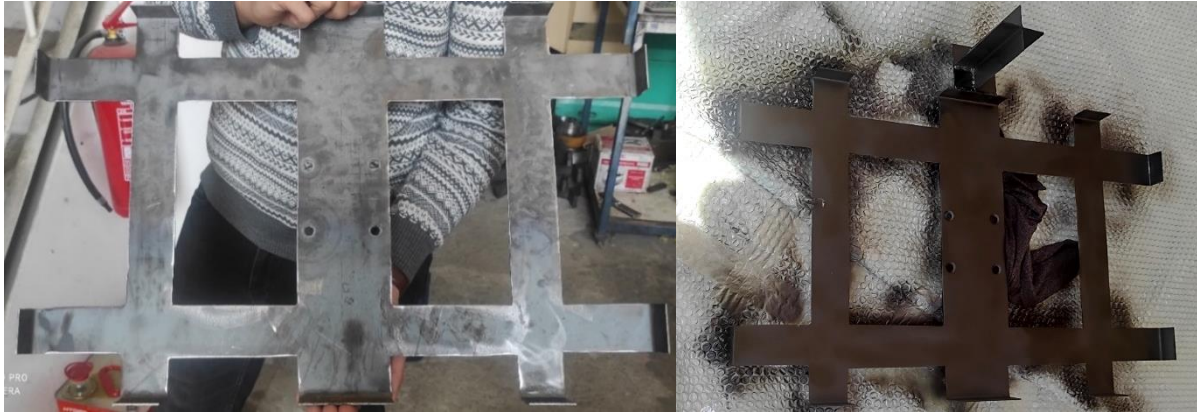
Figure 5. Solar panel holder apparatus
