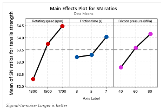
Figure 12. Main effects plot for S/N ratios of tensile strength.
