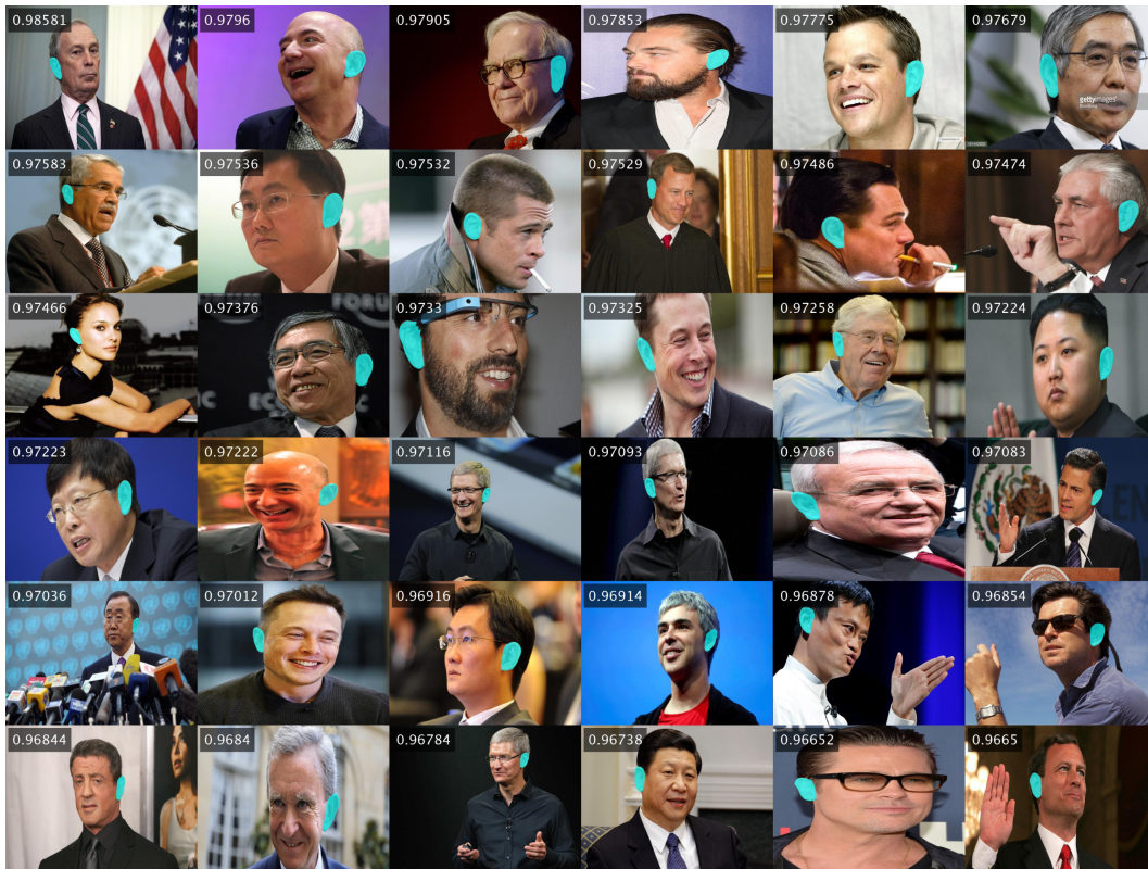
Fig. 2. Our ear segmentation results for the test images in the AWE dataset (with highest IoU scores).
