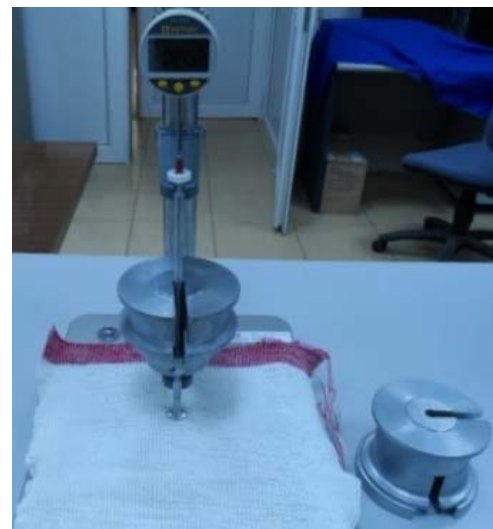
Figure 4. The thickness gauge and its additional weights
