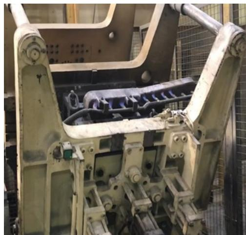
**Figure 11.3.** The tilt casting machine rotates 180 degrees.
