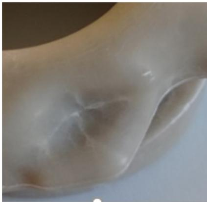
**Figure 5.** Salt core exterior surface crack.
