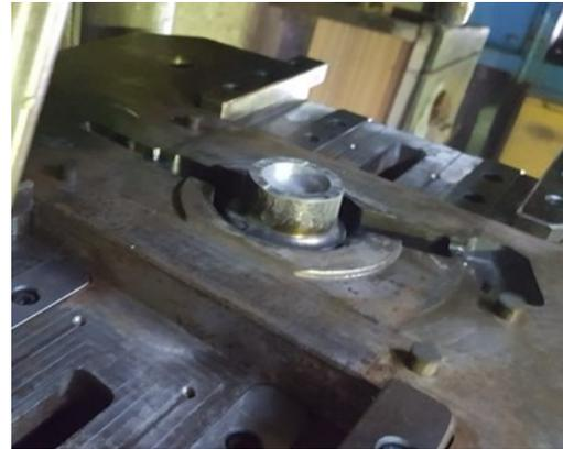
**Figure 7.** Mold inner diameter core insertion
