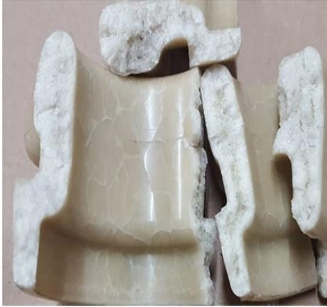
**Figure 9.** Inside view of salt core.
