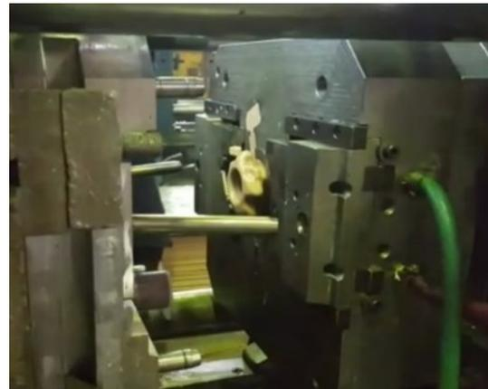
**Figure 3.** Salt core injection molding
