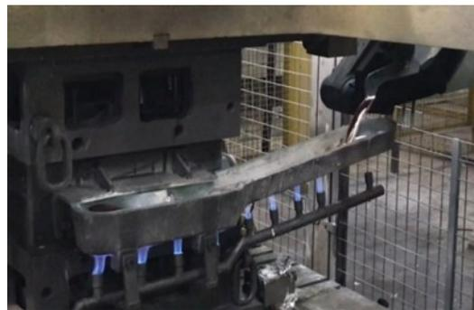
**Figure 11.2.** Tilt casting ladle.
