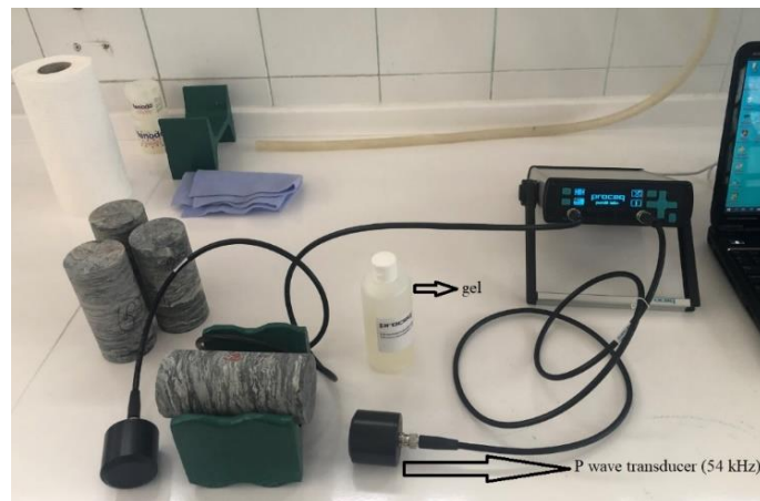
Figure 7. P wave experiment set-up.
