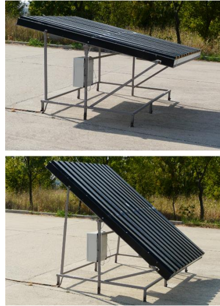
Figure 4. The 5 m 2 experimental setup used for roof ventilation measurements
