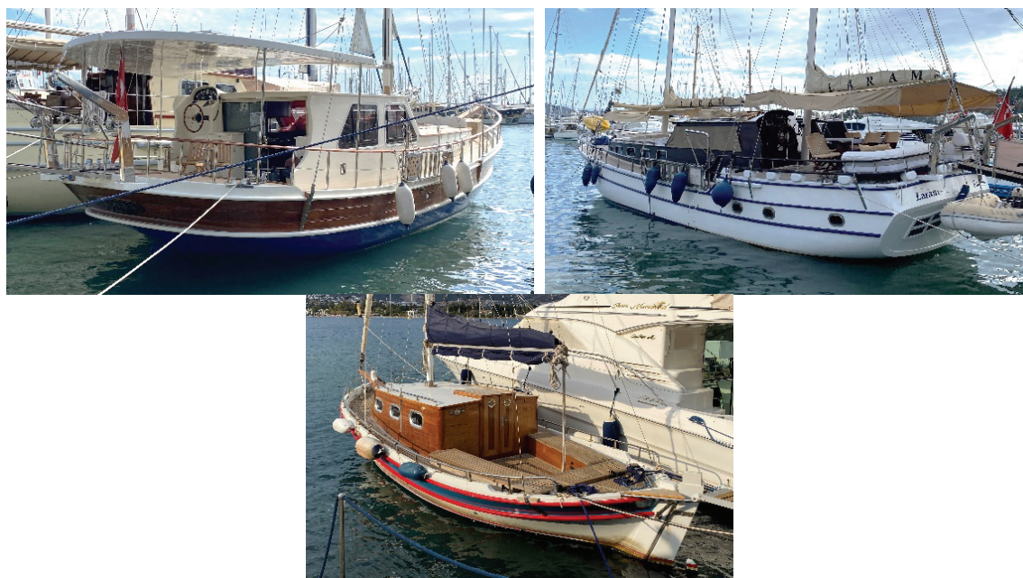
Figure 1. A Bodrum Gulet with round stern (top-left), transom stern (top-right), and a tirhandil (below)
