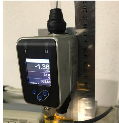
Figure 6. Flow Meter Connection
