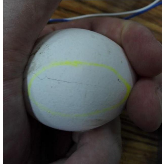
Figure 14 Image of micro-cracked egg under compression
