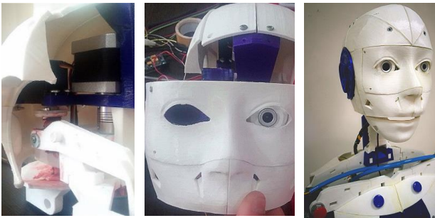
Figure 3. InMoov open source humanoid robot head design
