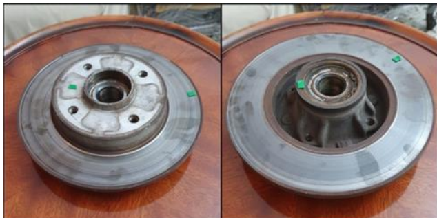
Figure 4. Front and rear view of disassembled brake disc
