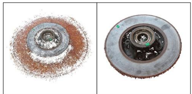
Figure 11. Sparse and dense point cloud data (rear)
