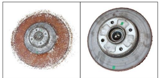
Figure 10. Sparse and dense point cloud data (front)
