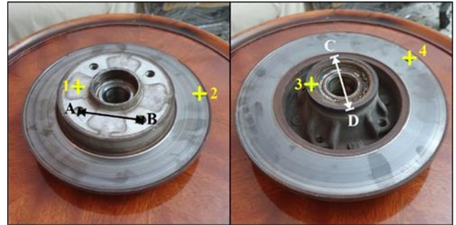
Figure 9. User tie points and scale constrains of the brake disc
