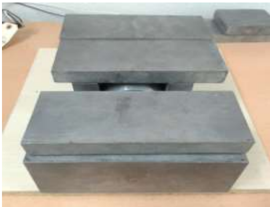
Figure 3. Side and up shielding plate
