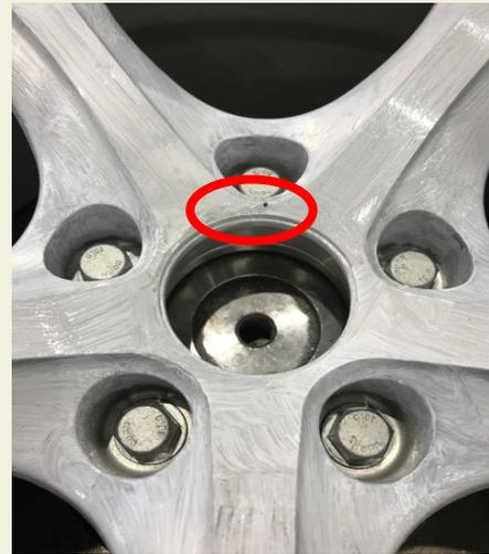
Figure 18. 2.00.000 cycles in long test
