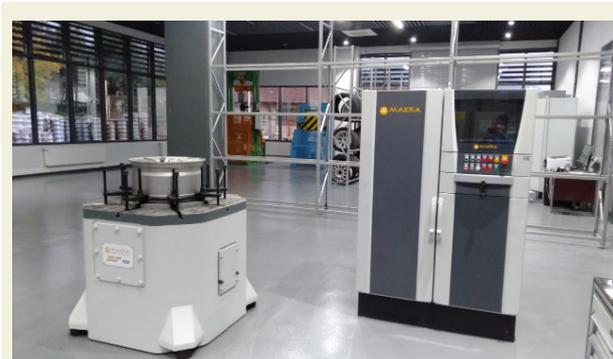
**Figure 5.** a)Scheme of the rotating bending fatigue test[5], b) testing machine
