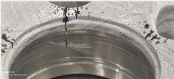
Figure 16. 2.500.000 cycles in short test [fail]
