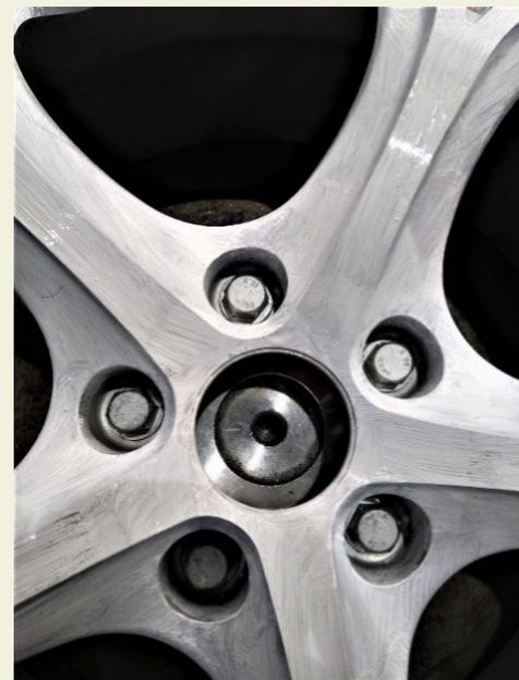
Figure 13. 200.000 cycles in short test
