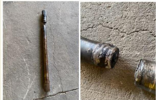
**Figure 4.** Damaged axle shaft
