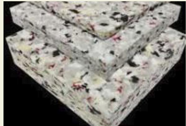
Figure 2. Acoustic material in sponge structure [72]
