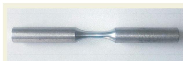
**Figure 2.** Fatigue specimen of Döktaş
