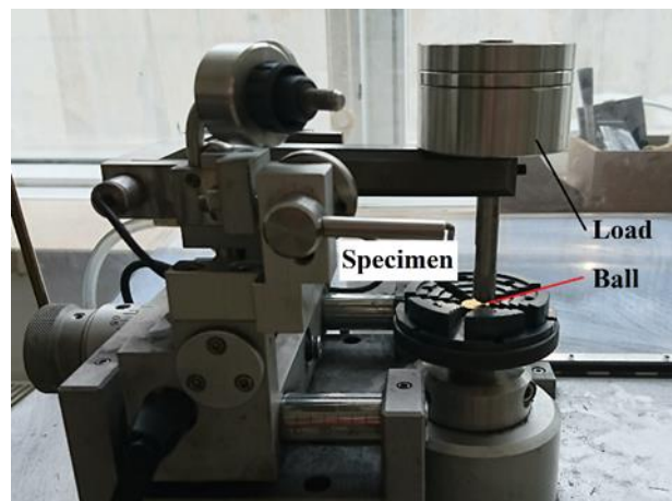
Figure 4. Ball-on-disc wear testing machine
