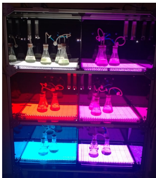
Figure 1. Arduino based computer controlled addressable RGB LED light system used for the experiments.
