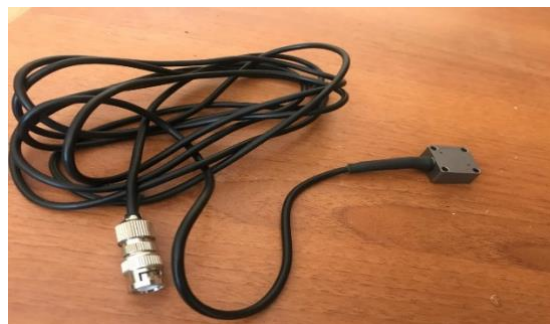
Figure 4. An example of the accelerometer sensor used
