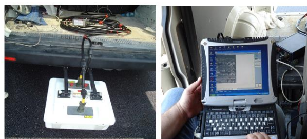
Figure 4. Installation of GPR antenna on vehicle and instant data transfer to PC.
