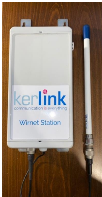
Figure 5- LoRaWAN gateway for data transmission
