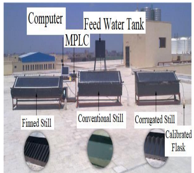
Figure 2. Photograph of conventional, corrugated and finned solar still [50].
