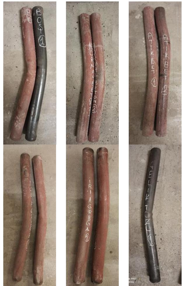
**Figure 5.** Test specimens after buckling
