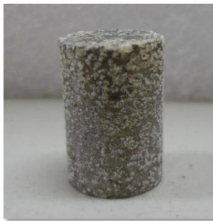
Figure 5. Image of the sample as a result of biuret formation from carbamide vapor
