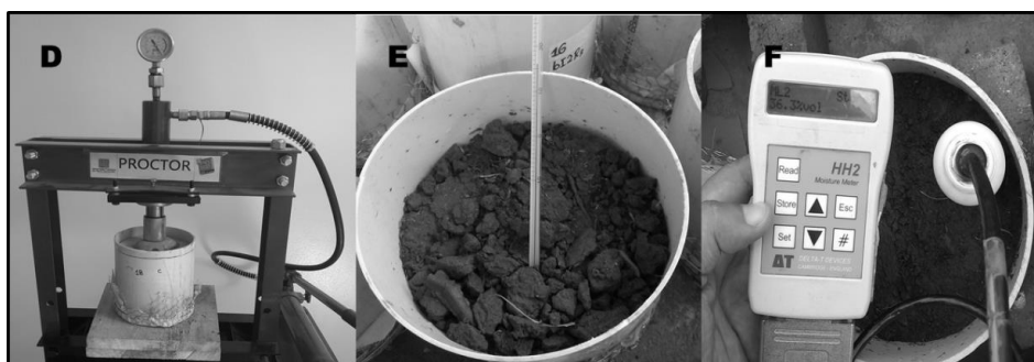
D: preparation of treatments with aeration <8% E: soil temperature monitoring with a Hg thermometer, F: soil moisture monitoring with a dielectric sensor.
