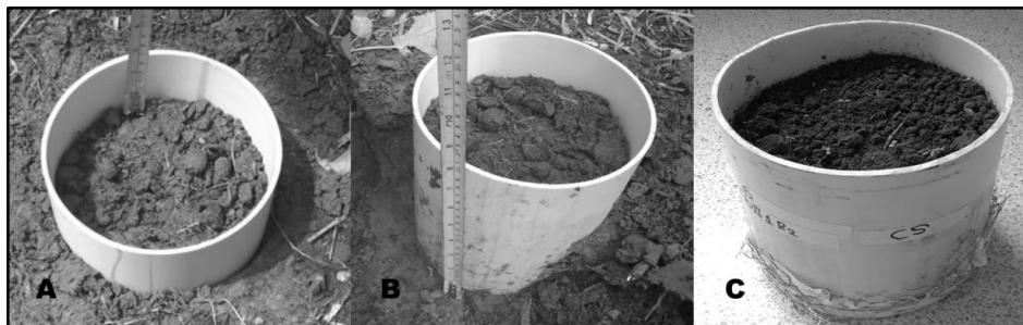
A: cylinder buried up to 15 cm deep with 5 cm edge. B: extraction of the cylinder with an undisturbed soil sample. C: cylinder prepared with canvas and mesh in its lower part. Figure 1. Images of the mesocosm design (experimental units) and construction process, with undisturbed soil at 15 cm depth in PVC cylinders of 18 cm in diameter and 20 cm in height.
