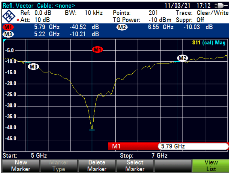
Figure 6. The screenshot of the VNA screen during the measurement of the manufactured antenna
