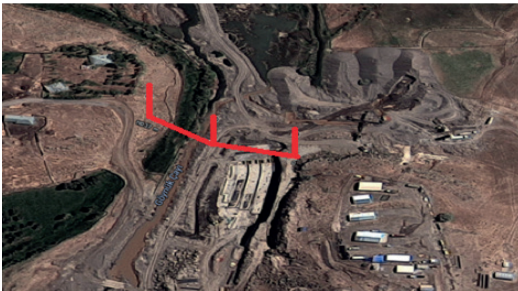
Figure 26. Dam-type reservoir for Saf HPP
