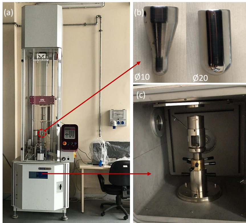
Figure 2. Drop weight test system: (a) Testing machine, (b) Impactors, (c) Clamping fixture
