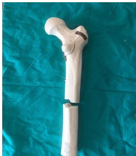
Figure 5. Transverse fractured bone model from the just distal of implant after axial loading
