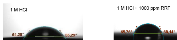
Figure 6. Contact angles of Cu surface after exposing to 1 M HCl solution in the absence and presence of 1000 ppm RRF
