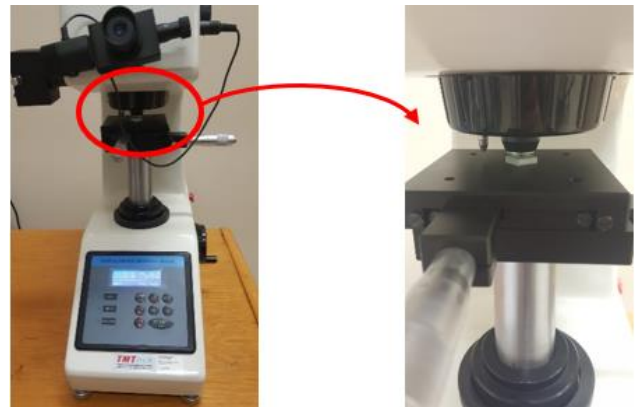
Figure 3. Digital microhardness testing device used in the present study
