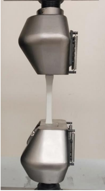
Figure 4. Tensile test sample and apparatus
