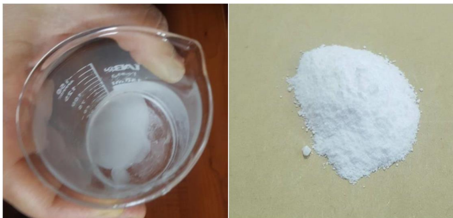
Figure 7. The gel product precipitated by the addition of acetone and the precursor powder obtained by drying the gel product [1].
