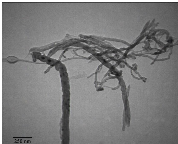
Figure 1. TEM micrograph of Pt@SWCNTs nano hybrid.
