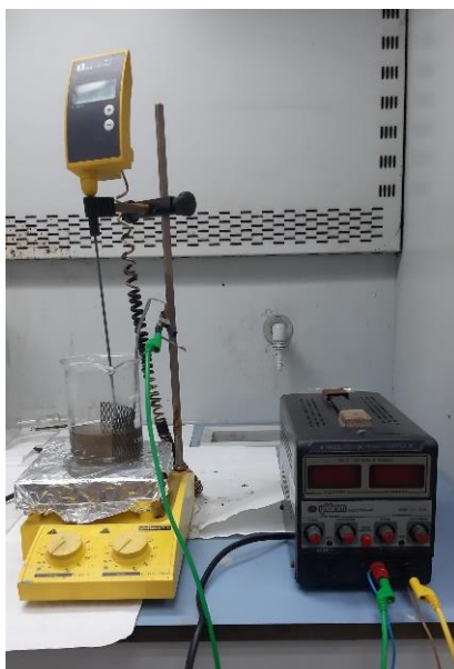
Figure 2. Electrolytic coating mechanism.
