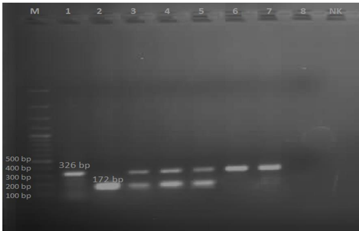
Figure 3. The image of the presence of sheep milk obtained by multiplex conventional PCR method in experimentally prepared goat milk. (M: 100 bp marker; 1: Goat milk (%100) (326 bp); 2: Sheep milk (%100) (172bp); 3: Goat and sheep milk (1%) mix; 4: Goat and sheep milk (2%) mix; 5: Goat and sheep milk (5%) mix; 6: Goat and sheep milk (0.1%) mixture; 7: Goat and sheep milk (0.5%) mixture; 8: Goat primer + sheep milk DNA; 9: Sheep primer + goat milk DNA).
