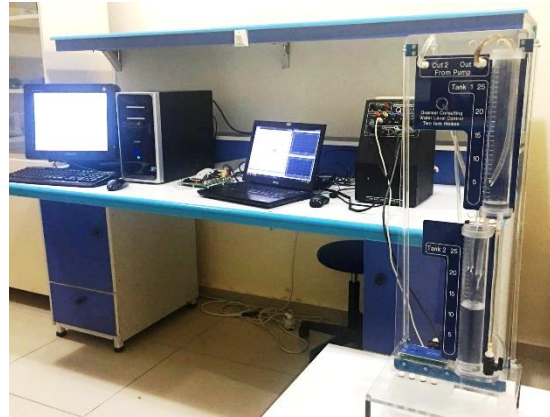
Figure 5. Quanser Coupled tank system setup
