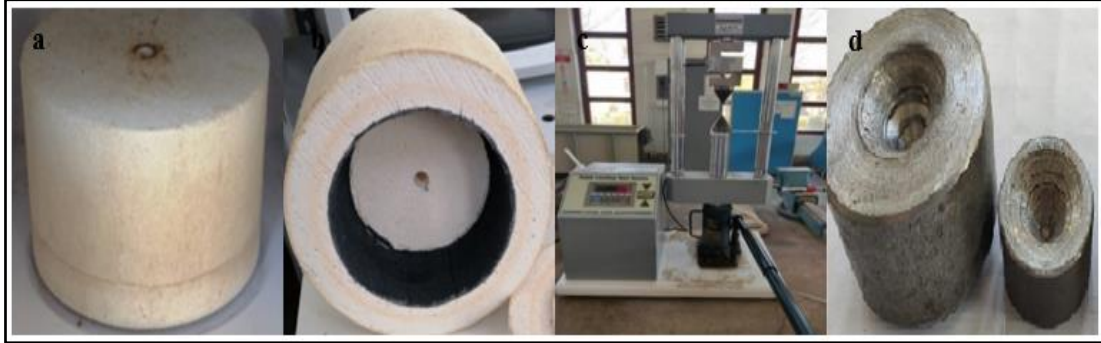
Figure 2. The photos of (a), microwave kiln (b), SiC coating inside the kiln (c) single point loading device (d) apparatus to spread the load uniformly
