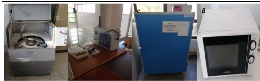
Figure 1. The photos of (a) ringed mill, (b) blaine device, (c) oven and (d) household microwave oven. Unit weight (UW) of the aggregates were calculated according to TS EN 1097-6 [19]. Fracture load of aggregates were determined by one point loading device using apparatus given in Fig. 2 to spread the load uniformly. One point loading device was preferred for precise measurement of the little crushing loads. All the reported results are the means of three samples. The crushing strength ( \sigma , kg/cm 2 ) for speherical aggregates are calculated by the equation 1 where: P: fracture load (kN), and X: the distance between loading points (mm) [20, 21]. SEM-EDX analyses on core and shell of the aggregates were conducted.
