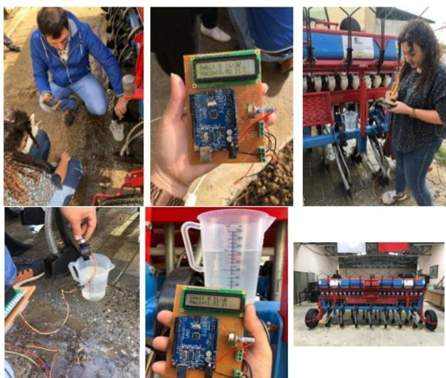
**Figure 2.** Calibration measurements taken for the designed system
