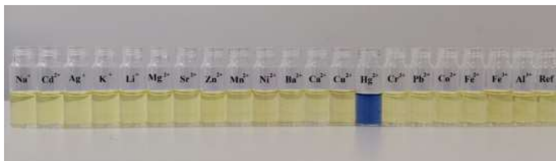
Fig. 2 Colorimetric change of ChL solution after addition of metal ions (1:1 metal-ligand stoichiometry in acetonitrile/water 10:1).
