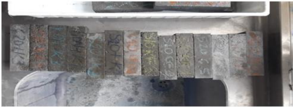
Fig. 3 Samples taken from curing pool
